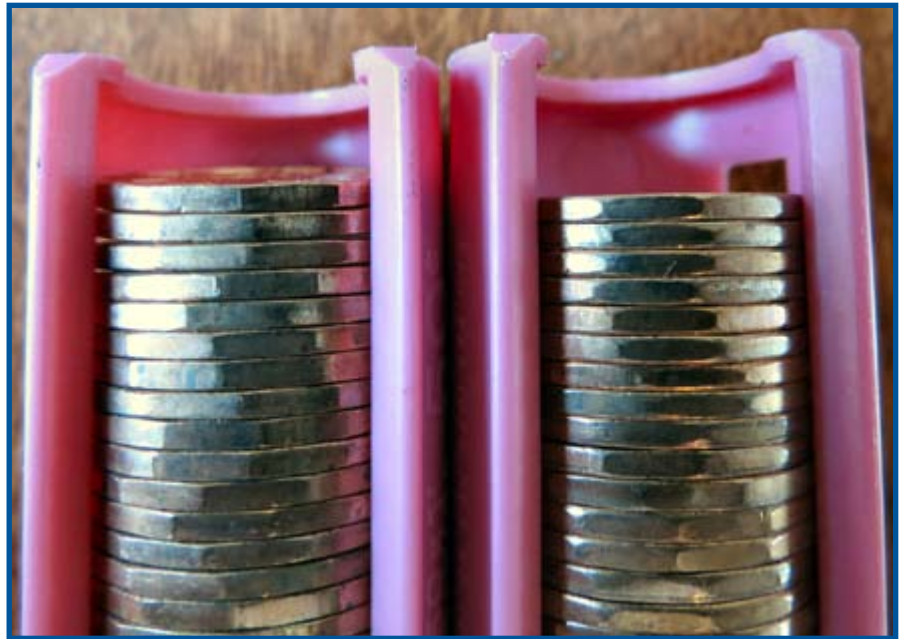
The Penny Pincher on the left is holding a roll of 50 uncirculated 1984 "pennies". The one on the right has 50 uncirculated 1982 "pennies". Neither is full, and the 1982 "pennies" are clearly thinner than the 1984 coins. Could these 1982 coins have been struck on leftover blanks originally intended for the thinner 1981 coins? Their weight tells no.
